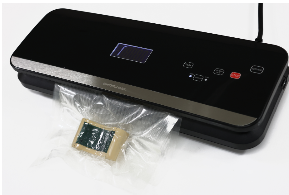
Figure 2 Vacuum sealing method. A specimen positioned on a working cast was sealed using a vacuum sealing device.
